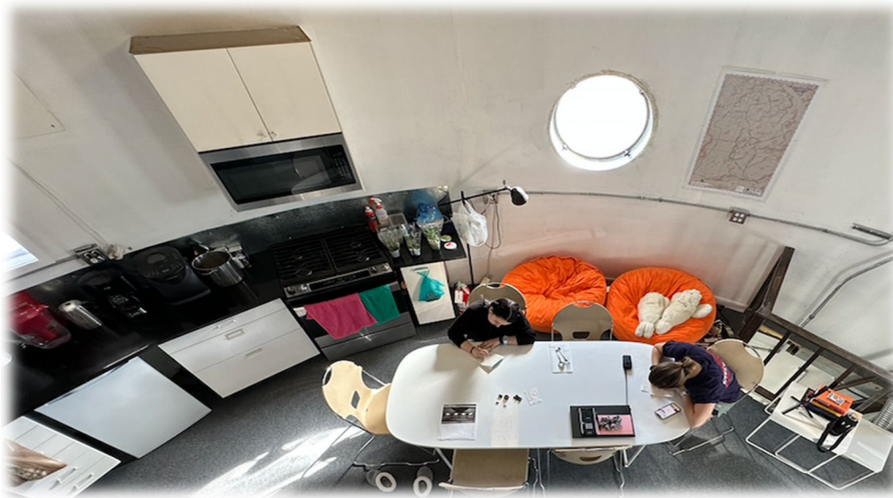
Fig. 3 A photograph of the crew's daily life illustrates that the microwave is mounted on the exterior wall of the common room of the habitat, which create opportunity for constant temperature fluctuation
