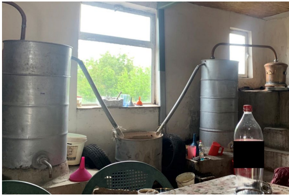
Fig. 5 Local legal facility for rakia distillation from the village of Belogradets, Varna county, Bulgaria. The stainless-steel cauldron has a fine copper net incorporated in it for neutralizing toxic by-products and bacterial contamination (Source authors' own photo)
