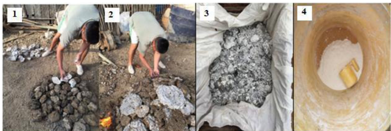
Fig. 6 Preparation of oyster lime. 1 Manure and shells placed on the ground. 2 A kind of mound is formed. 3 Shells bathed in water and covered with a kitchen tablecloth. 4 Lime powder, by Efrén Silva (the first author of this article), Guayaquil, Ecuador
